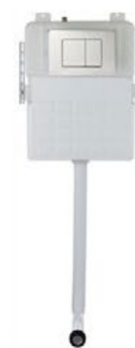
TA00003 Concealed Cistern for Wall-Hung Toilet INSTALL SIZE: 480x120x1130mm FLUSH VOLUME: 3L-6L Operation mode Pneumatic push button control
