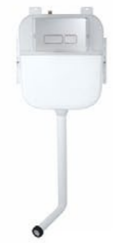
TA00006 Concealed Cistern for back to wall toilet INSTALL SIZE: 500x95x1140mm FLUSH VOLUME: 3L-6L Operation mode Pneumatic push button control
