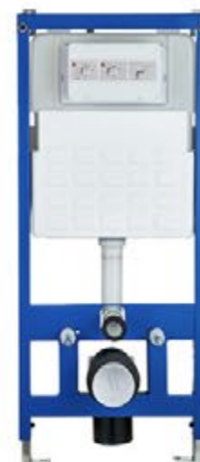
TA00001 Concealed Cistern for Wall-Hung Toilet INSTALL SIZE: 500x120x1140mm FLUSH VOLUME: 3L-6L Operation mode Pneumatic push button control
