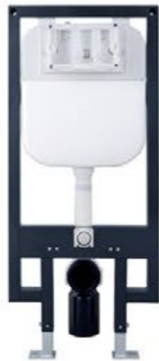
TA00012 Concealed Cistern INSTALL SIZE: 500x120x1140mm FLUSH VOLUME: 3L-4.5L Operation mode Pneumatic push button control
