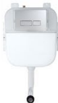
TA00014 Concealed Cistern INSTALL SIZE: 460x95x770mm FLUSH VOLUME: 3L-4.5L Operation mode Pneumatic push button control
