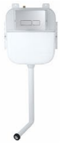
TA00013 Concealed Cistern INSTALL SIZE: 460x95x1100mm FLUSH VOLUME: 3L-4.5L Operation mode Pneumatic push button control
