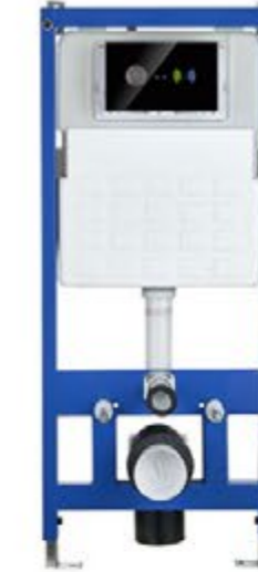
TA00029 Sensor Operated Concealed Cistern INSTALL SIZE: 500x120x1140mm FLUSH VOLUME: 3L-6L Operation mode Pneumatic push button control
