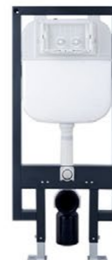
TA00005 Concealed Cistern for Wall-Hung Toilet INSTALL SIZE: 500x95x1140mm FLUSH VOLUME: 3L-6L Operation mode Pneumatic push button control
