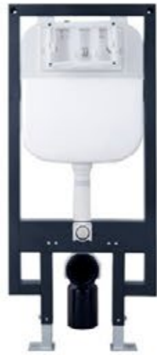
TA00009 Concealed Cistern INSTALL SIZE: 500x120x1140mm FLUSH VOLUME: 3L-6L Operation mode Pneumatic push button control
