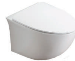
EP0203 -Wall Hung -Soft close Seatcover -"S" Trap -Rough-in 180mm -3\4.5L Flush Volume -Dimensions 520x370x360mm
