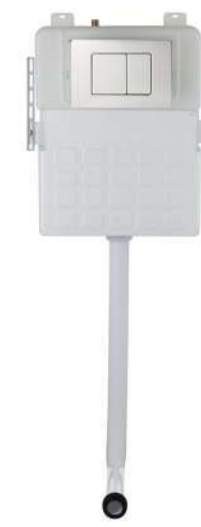
PBTA0070 Concealed Cistern Install size: 480x120x1130mm. flush volume : 3L-6L Operation mode: Pneumatic push button control.
