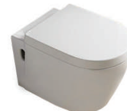
EP0238 -Wall-Hung -Soft close Seatcover -"P" Trap -Rough-in 180mm -3\4.5L Flush Volume -Dimensions 555x360x360mm
