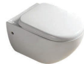
EP0202 -Wall-Hung -Soft close Seatcover -"P" Trap -Rough-in 180mm -3\4.5L Flush Volume -Dimensions 550x380x350mm
