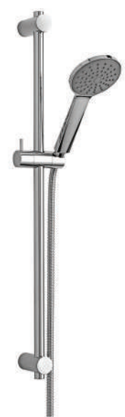
ZSALNF00433 Sliding rail shower set Complete With:- •Metal rod Ø20,5 x L.730 mm •ABS hand shower, single spray, Ø105 mm •Double interlock twist-free metal flexible hose 1500 mm
