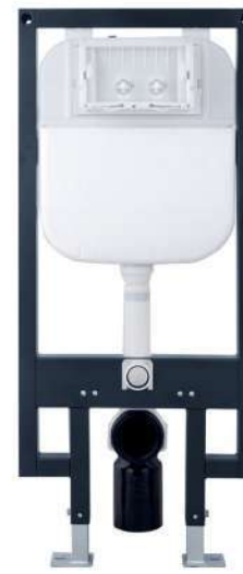
PBTA0072 Concealed Cistern Install size: 500x95x1140mm. flush volume : 3L-6L Operation mode: Pneumatic push button control.
