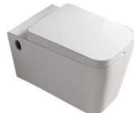
SWCEP0017 -Wall-Hung -Soft close Seatcover -"P" Trap -Rough-in 250mm -3\4.5L Flush Volume -Dimensions 570x350x330mm
