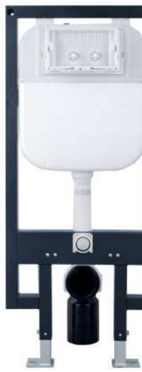
PBTA0074 Concealed Cistern Install size: 500x95x1140mm. flush volume : 3L-4.5L Operation mode: Pneumatic push button control.
