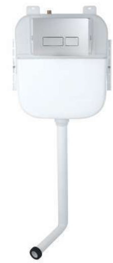
PBTA0077 Concealed Cistern Install size: 460×95×1100mm. flush volume : 3L-6L Operation mode: Pneumatic push button control.
