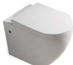
EP0201 -Wall Hung -Soft close Seatcover -"S" Trap -Rough-in 180mm -3\4.5L Flush Volume -Dimensions 490x340x360mm
