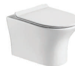
SWCEP0003 -Wall Hung -Soft close Seatcover -"S" Trap -Rough-in 180mm -3\4.5L Flush Volume -Dimensions 490x340x360mm
