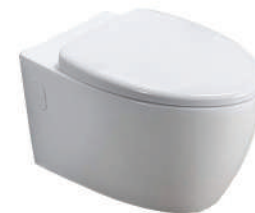
EP0215 -Wall-Hung -Soft close Seatcover -"P" Trap -Rough-in 180mm -3\4.5L Flush Volume -Dimensions 570x390x355mm
