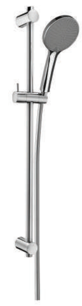
ZSALNF00432 Sliding rail shower set Complete With:- •Metal rod Ø20,5 x L.730 mm •ABS hand shower, three-spray functions, Ø110 mm •Double interlock flexible hose 1500mm
