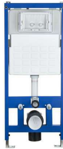
PBTA0082 Concealed Cistern Install size: 500×120×1140mm. flush volume : 3L-6L Operation mode: Pneumatic push button control.
