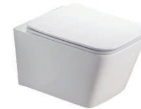
SWCEP0019 -Wall-Hung -Soft close Seatcover -"P" Trap -Rough-in 250mm -3\4.5L Flush Volume -Dimensions 550x350x345mm
