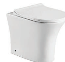
SWCEP0002 -Back To Wall -Soft close Seatcover -"S" Trap -Rough-in 250mm -3\4.5L Flush Volume -Dimensions 520x340x400mm
