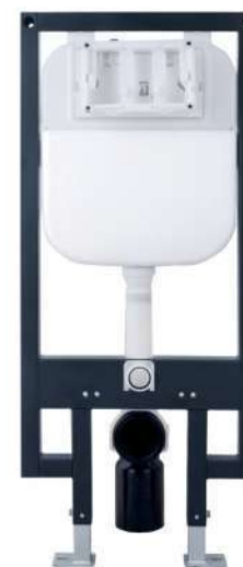
PBTA0079 Concealed Cistern Install size: 500×120×1140mm. flush volume : 3L-4.5L Operation mode: Pneumatic push button control.
