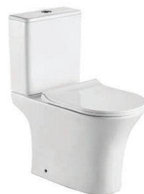
SWCEP0001 -Close-Coupled -Soft close Seatcover -"S" Trap -Rough-in 250mm -3\4.5L Flush Volume -Dimensions 650x340x770mm
