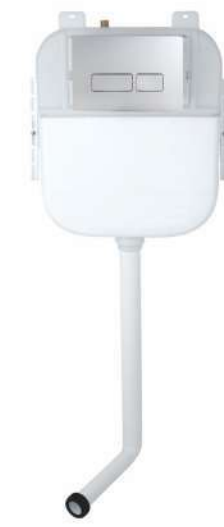
PBTA0073 Concealed Cistern Install size: 500x95x1140mm. flush volume : 3L-6L Operation mode: Pneumatic push button control.
