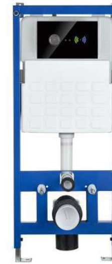
PBSTA0082 Sensor Operated Concealed Cistern Install size: 500×120×1140mm. flush volume : 3L-6L Operation mode: Pneumatic push button control.
