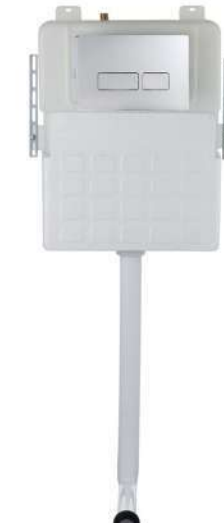
PBTA0083 Concealed Cistern Install size: 500×120×1140mm. flush volume : 3L-6L Operation mode: Pneumatic push button control.
